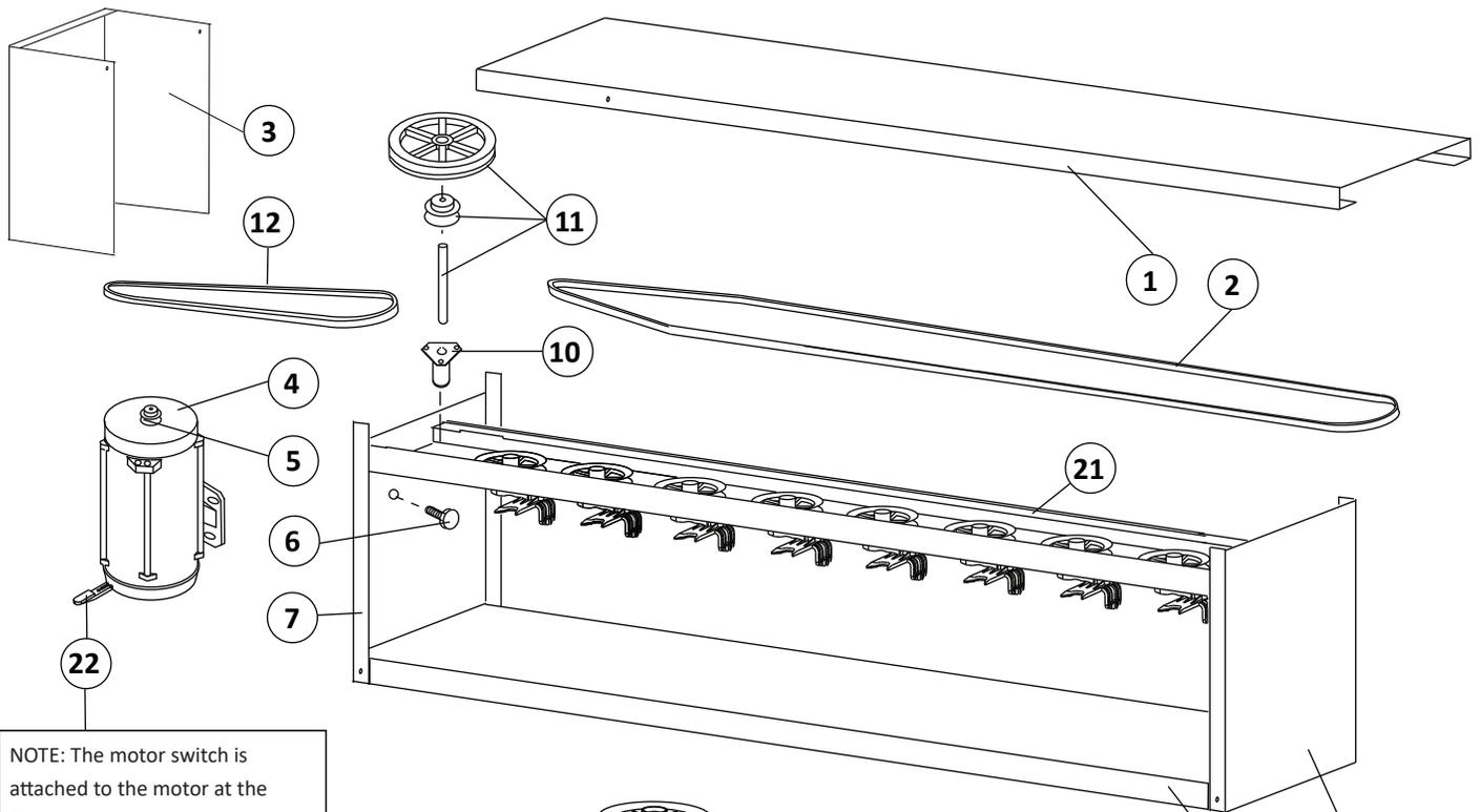
NOTE: The motor switch is attached to the motor at the factory. It is located under the left side of the motor guard.
