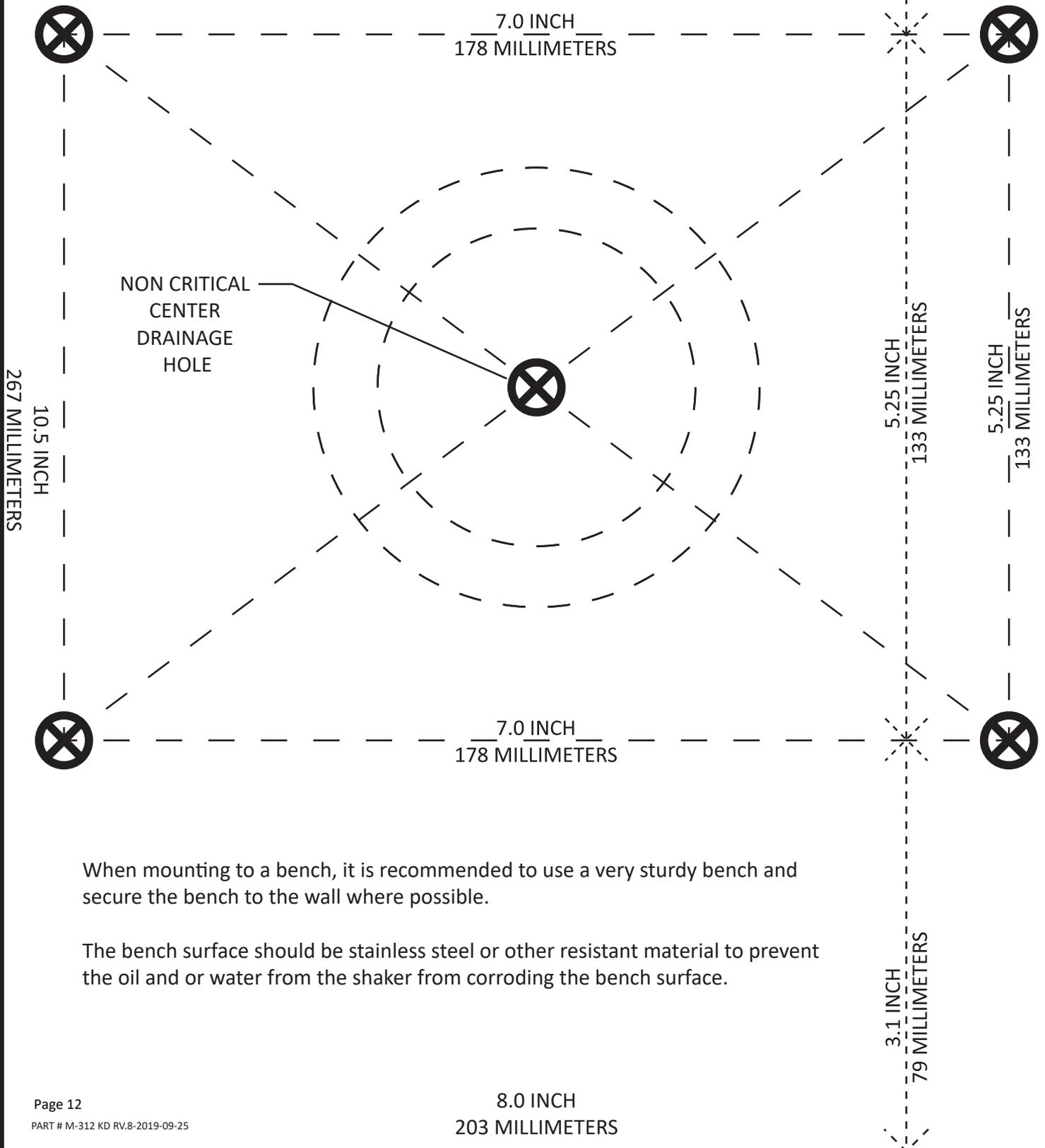
When mounting to a bench, it is recommended to use a very sturdy bench and secure the bench to the wall where possible.
