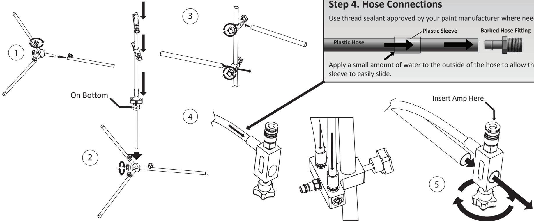
Step 1: Assemble the three feet onto the base hub.
