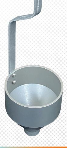
Do not use a hard cleaning device to clean the orifice at the bottom of the cup, as the size of this opening is critical to the accuracy of the metering control. Any modification of this orifice will affect the accuracy of this viscosity cup.
