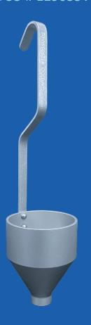
The DIN 4 viscosity cup is used to measure the viscosity or thickness of a liquid after reduction and additives are mixed together while it is prepared for spraying. Besides reduction, the thickness of the paint can also be a function of product temperature. The warmer the product the thinner it will be.
